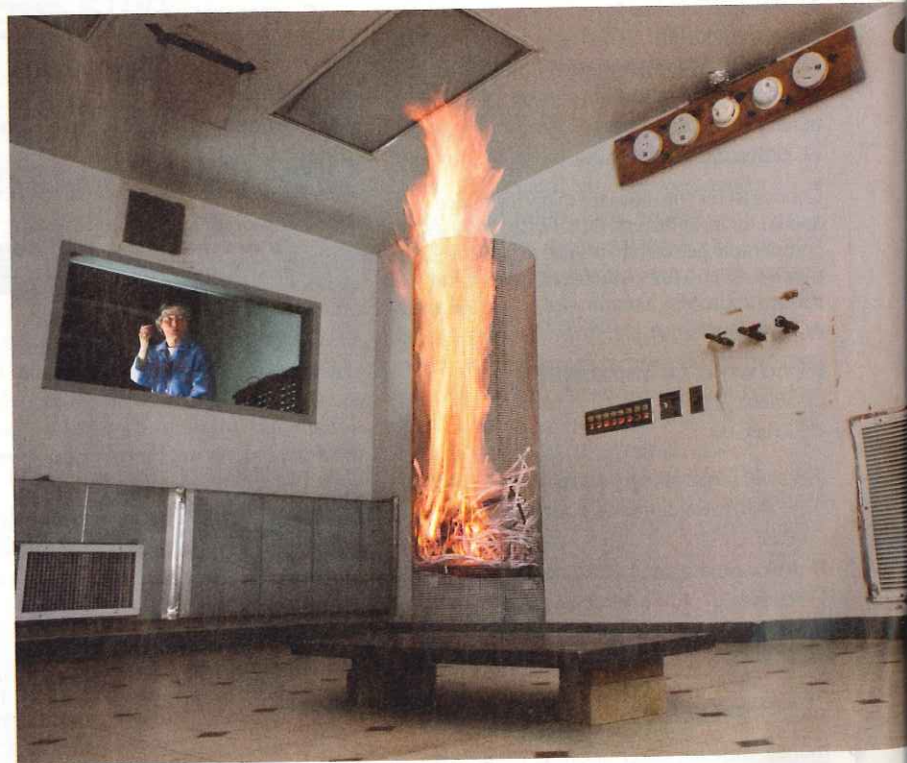
BURN NOTICE Our flash-fire test tracks how long it takes for the smoke detectors, upper right, to set off an alarm. Senior project leader Deborah Wallace oversees testing in a sealed lab.
